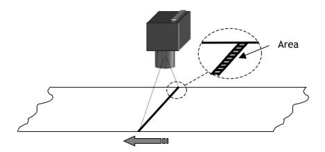
Fig. 8. The principle of line scan.
